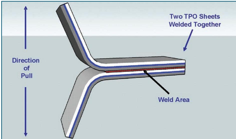
Figure 3 – TPO sheets welded together prior to T-peel testing for lamination strength.
